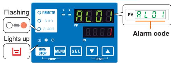
Alarm codes can be used for the notification of upcoming recommended maintenance. The codes notify you when it's time to check the pump and fan motor. Helpful for facility maintenance
